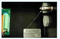
•UNUSED CABLE GLANDS MUST BE BLOCKED. •THIS UNIT SHOULD PREFERRABLY ALWAYS BE POWERED TO AVOID CONDENSATION
