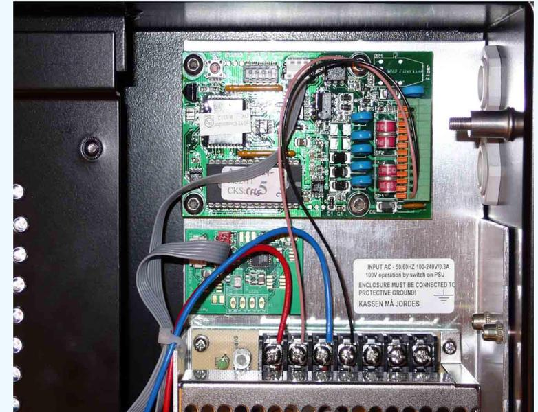
Check that the ground terminal on the power supply is connected to your system safety ground. Note that you may alternatively use the outside ground terminal (M6x15 screw)
